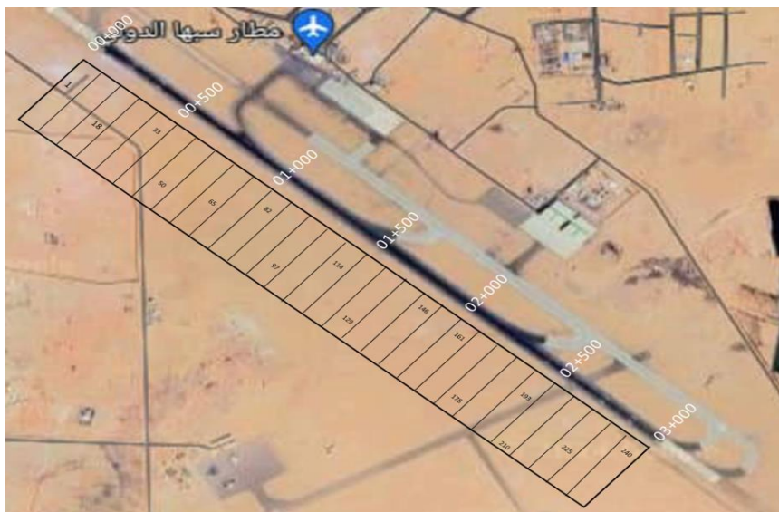
Figure (2). Satellite image of Sebha Airport, divided into 30 segments and sample units
